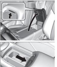
Slide the armrest to the rearmost position. Pull the handle to open the console compartment.
