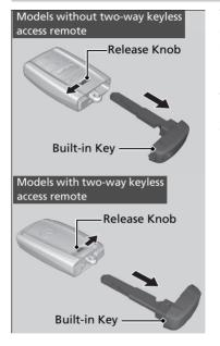
The built-in key can be used to lock/unlock the doors when the keyless access remote battery becomes weak and the power door lock/ unlock operation is disabled.
