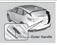
When all the doors are unlocked, the tailgate is unlocked.
