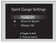
Press the right selector wheel when you select the **Sport Gauge Settings** on the multiinformation display. Roll the right selector wheel to select the setting and press it.
