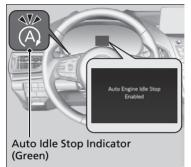
The engine then restarts once the vehicle is about to move again, and the indicator (green) goes off.
