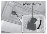
If you need to talk to the AcuraLink operator in a situation where no airbag has deployed, you can manually connect to them by pressing the **ASSIST** button with the power mode in ACCESSORY or ON.
