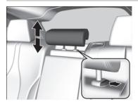
A passenger sitting in a center back seating position should adjust the height of their head restraint to an appropriate position before the vehicle begins moving. **To raise the head restraint:** Pull it upward. **To lower the head restraint:** Push it down while pressing the release button.
