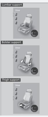
Press the mode selector up or down to select the lumbar support adjustment mode, bolster support adjustment mode or thigh support adjustment mode.
