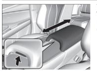
The console lid can be used as an armrest. **To adjust:** Pull the handle and slide the armrest to desired position.
