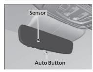
When you are driving after dark, the automatic dimming rearview mirror and automatic dimming power door mirrors reduce the glare from headlights behind you, based on inputs from the mirror sensor. Press the auto button to turn this function on and off. When activated, the auto indicator comes on.
