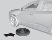
**9.** Place the compact spare tire (wheel side up) under the vehicle body, near the tire that needs to be replaced.
