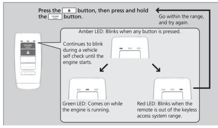
The engine runs for up to 10 minutes without you starting the vehicle. To extend the run time for another 10 minutes during the first run, press the <u>a</u> button, then press and hold the <u>record</u> button.
