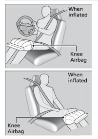
The driver's and front passenger's knee airbag deploy at the same time as the driver's and front passenger's airbag respectively.
