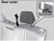
Front Release Button **To raise the head restraint:** Pull it upward. **To lower the head restraint:** Push it down while pressing the release button.
