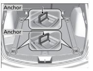
The tie-down anchors on the cargo area floor can be used to install a net for securing items.
