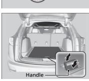
**1.** Push the rear edge of the handle on the floor lid and open the lid.
