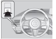
Turn the headlights on and press the headlight washer button to operate. The headlight washers also operate when you turn the windshield washers for the first time after the power mode is set to ON.
