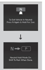
If the **ENGINE START/STOP** button is pressed after car wash mode has been activated, the power mode will change to ACCESSORY and a message will be displayed on the multiinformation display.
