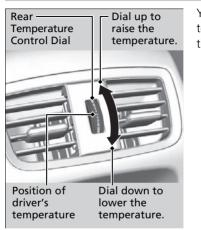
You can set the rear passenger compartment temperature different than the driver's, using the rear temperature control dial.
