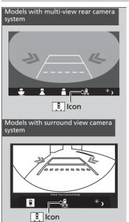
You can switch the system on and off using the audio/information screen.
