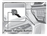
To open or close the power tailgate, press the power tailgate button for about one second.
