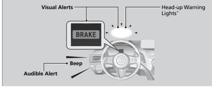
You can change the distance (**Long/Normal/Short**) between vehicles at which the system's earliest collision alert will come on through audio/information screen setting options.
