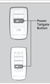
Press the power tailgate button for more than one second to operate when the power mode is in VEHICLE OFF (LOCK).
