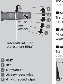
The windshield wipers and washers can be used when the power mode is in ON.
