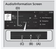
(A): Shows how much time the replayed segment is behind the real-time broadcast
