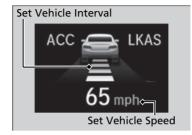
When ACC with Low Speed Follow starts operating, the vehicle icon, interval bars and set speed appear on the multi-information display.
