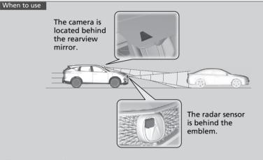
Vehicle speed for ACC with Low Speed Follow: A vehicle is detected ahead within ACC with Low Speed Follow range – ACC with Low Speed Follow operates at speeds up to 90 mph (145 km/h).
