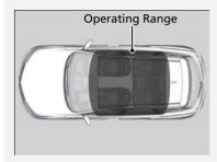
You can start the engine when the keyless access remote is inside the vehicle
