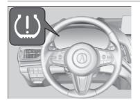
Monitors the tire pressure while you are driving. If your vehicle's tire pressure becomes significantly low, the low tire pressure/TPMS indicator comes on and a message appears on the multi-information display.
