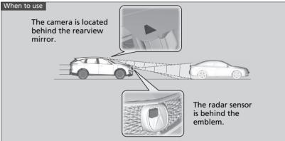
The system starts monitoring the roadway ahead when your vehicle speed is about 3 mph (5 km/h) and there is a vehicle in front of you.
