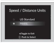
Enables you to show another unit on the multi-information display, head-up display\* and audio/information screen and set the displayed measurements to read in either miles and km, mph and km/h.
