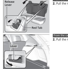
From the rear door side 2. Pull the release lever.
