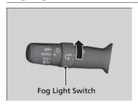
When the low beam headlights are on, turn the fog light switch on to use the fog lights.
