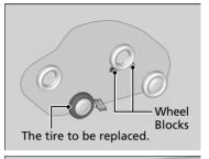
**8.** Place a wheel block or rock in front and rear of the wheel diagonal to the flat tire.
