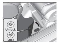
The front floor mats hook over floor anchors, which keep them from sliding forward. To remove a mat for cleaning, turn the anchor knobs to the unlock position. When reinstalling the mat after cleaning, turn the knobs to the lock position.
