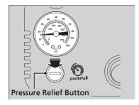
9. Press the pressure relief button until the gauge returns to 0 psi (0 kPa).10. Repackage and properly stow the kit.
