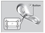
The gear position changes to  $\boxed{P}$  when you press the  $\boxed{P}$  button while the vehicle is parked with the power mode in ON. The indicators on the sides of the  $\boxed{P}$  button come on.
