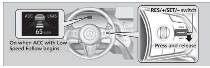
When driving at about 25 mph (40 km/h) or above: Take your foot off the pedal and press down the **RES/+/SET/–** switch when you reach the desired speed. The moment you release the switch, the set speed is fixed, and ACC with Low Speed Follow begins.
