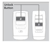
**To open:** Press the unlock button, and then within 10 seconds, press it again and hold it.
