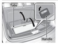
Pull the handle and remove the tabs to open the cargo floor lid.
