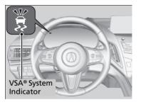
When VSA<sup>®</sup> activates, you may notice that the engine does not respond to the accelerator. You may also notice some noise from the hydraulic brake system. You will also see the indicator blink. Wehicle Stability Assist<sup>™</sup> (VSA<sup>®</sup>), aka Electronic Stability Control (ESC), System
