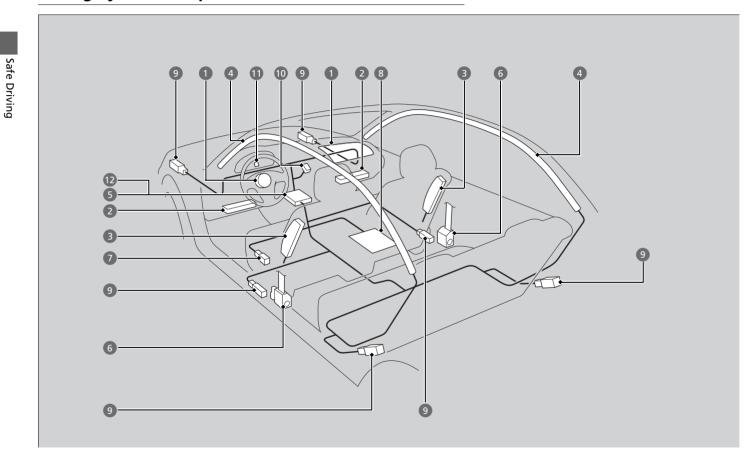
The front, driver's knee, front passenger's knee, front side, and side curtain airbags are deployed according to the direction and severity of impact. Both side curtain airbags are deployed in a rollover. The airbag system includes:
