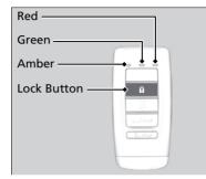
You can remotely check if your vehicle's doors are all locked or any are unlocked using the keyless access remote from extended distances.
