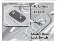
Press the master door lock switch in as shown to lock or unlock all the doors, tailgate and fuel fill door.
