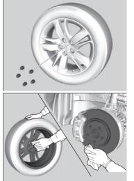
1. Remove the wheel nuts and flat tire.
