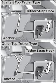
A tether anchor point is provided behind each rear seating position.
