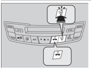
Pressing the result button turns the air conditioning system on and automatically switches the system to fresh air mode.
