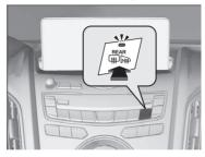
The rear defogger and heated door mirrors automatically switch off after 10-30 minutes depending on the outside temperature.
