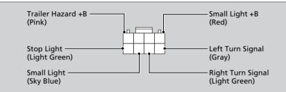
Your trailer lighting connector is located behind the left side panel in the cargo area. Each pin's purpose and wiring color code are shown in the image.
