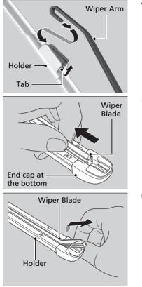
4. Press up on and hold the tab, then slide the holder off the wiper arm.
