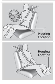
The knee airbag for the driver and the one for the front passenger are housed under the steering column and the glove box respectively.
