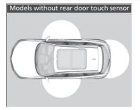
When you carry the keyless access remote, you can lock/unlock the doors, fuel fill door, and open the tailgate.
