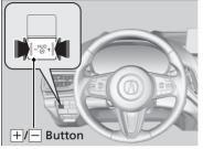
When the power mode is in ON, you can use the |+|/| button to adjust head-up display brightness. **Brighten:** Press the + button. **Dim:** Press the — button.
