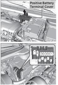
Remove the cover on the  $\oplus$  terminal (as shown).
