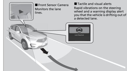
When you operate the turn signals to change lanes, the system is suspended, and resumes after the signals are off.
