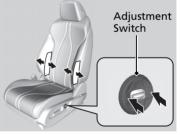
To adjust the lumbar support: Press the top: To move the lumbar support up. Press the bottom: To move the lumbar
