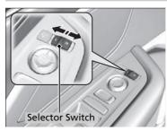
If activated, either side door mirror automatically tilts downward when you put the transmission into  $[\mathbf{R}]$ ; this improves closein visibility on the selected side of the vehicle when backing up. The mirror automatically returns to its original position when you take the transmission out of  $[\mathbf{R}]$ .
