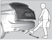
Use a forward and back kicking motion under the center of the rear bumper to open or close the power tailgate while carrying the keyless access remote.
