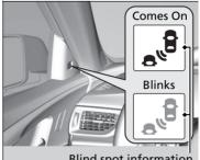
Blind spot information System Alert Indicator Blind spot information System Alert Indicator: Located near the pillar on both sides.
