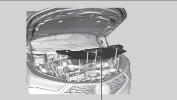
Remove the Engine Compartment Cover
