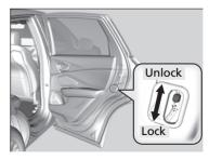
Slide the lever in the rear door to the lock position, and close the door.
