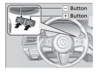
When the parking lights are turned on and the power mode is in ON, you can use the + or - button to adjust instrument panel brightness. **Brighten:** Press the + button. **Dim:** Press the - button.
