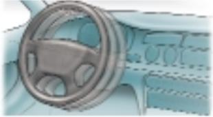
A collapsible steering column, smooth or recessed controls, and energy-absorbing materials help reduce crash injuries.
