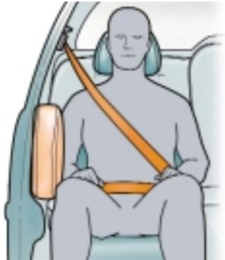
Side airbags provide a cushion to help protect the driver's or front passenger's upper torso.
