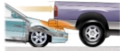
When a car underrides another vehicle at relatively low speed, the impact usually involves only crushable body parts, and the front airbags rarely deploy.
