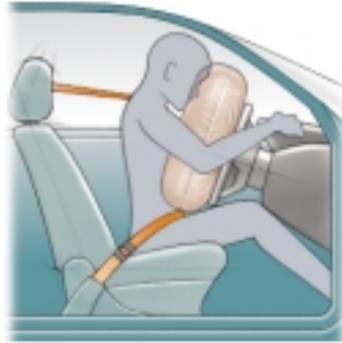
When sensors detect a moderate-to-severe frontal impact, the airbags instantly inflate to help protect the heads and chests of front-seat occupants.
