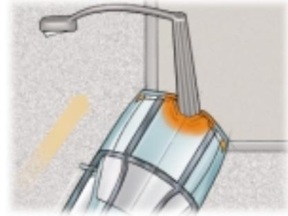
Crashing head-on into a pole or tree is less likely to cause airbag deployment than if you strike the object off-center near the car's strong metal framework.
