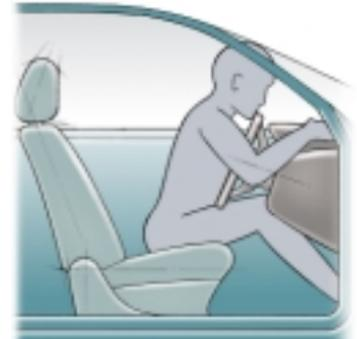
Without a seat belt or an airbag, the occupant will continue forward at 48 kph until they strike the car's interior, and potentially suffer very serious injuries.
