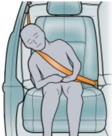
If sensors detect that the front passenger is a child or small adult, and the passenger has leaned into the side airbag's deployment path, the airbag will automatically turn off.
