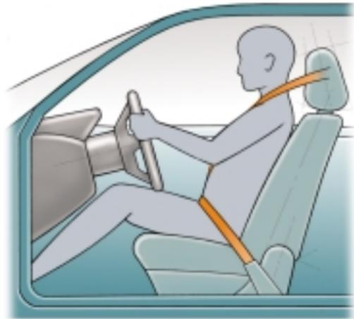
Wearing a seat belt, and sitting upright, at least 25 cm (10 inches) back from the steering wheel or dashboard, reduces the chance of injuries caused by an inflating front or side airbag.
