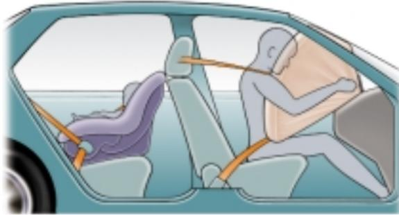
To avoid the possibility of an infant being seriously injured or killed by an inflating front airbag, a rear-facing child seat should always be secured in the back seat, never in the front.
