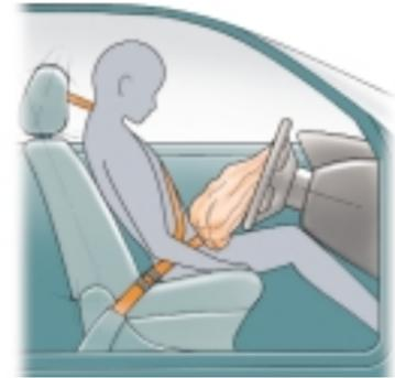
After inflating, the airbags immediately deflate so they won't interfere with the driver's visibility or ability to steer or operate other controls.
