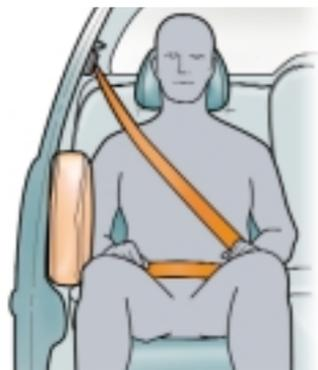
If the impact is moderate-to-severe, the side airbag on the impact side will inflate from the outer seat-back bolster to help protect the occupant's upper torso.
