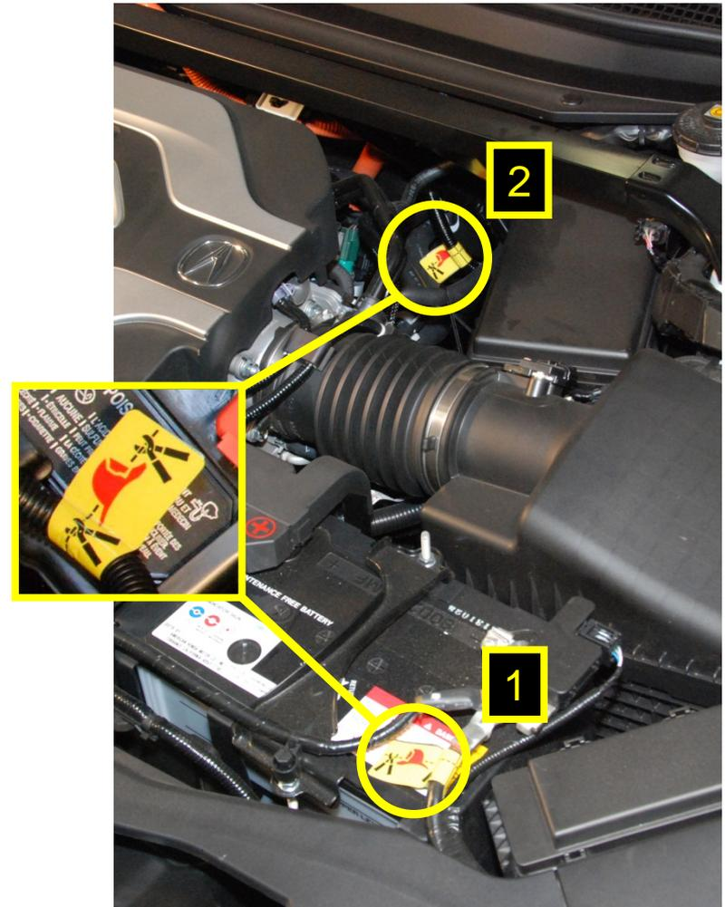
*Cut the negative 12V battery cable and then cut the DC to DC Converter cable.*
