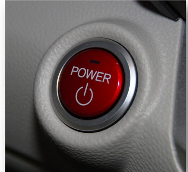
*Push and hold the start/stop button for 3 seconds*
