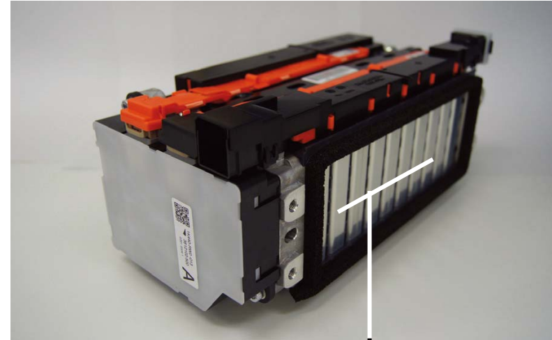
One of Four Battery "Stacks"
