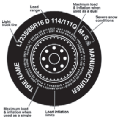
Figure 4: Typical Light Truck Tire Markings
