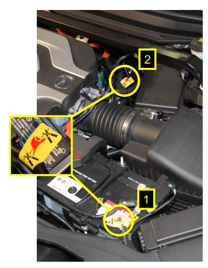
Cut the negative 12V battery cable and then cut the DC to DC Converter cable.
